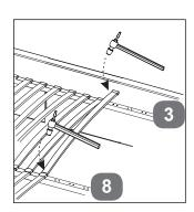
Fix slats (10) to double plastic cap (12) on one end, fix single caps (11) to each end, then connect onto centre support bar (8) & metal support rails of side rails (3) by gently tapping lugs down into the holes.
